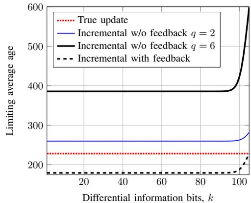
Figure 7. This plot shows the variation of the limiting average age as the number of bits needed to represent incremental information bits,  $k$ , grows. We have chosen the number of information bits  $m = 105$ , in each codeword of length  $n = 120$  bits. The erasure probability of the *iid* bit-wise binary symmetric channel is taken as  $\epsilon = 0.1$ .
