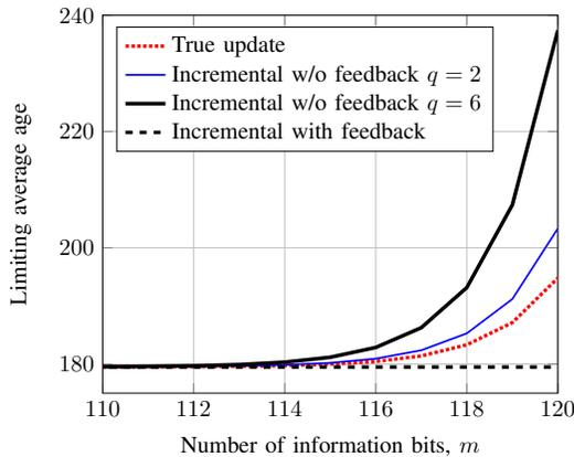
Figure 5. This plot shows the variation of limiting average age as the number of information bits  $m$  grows. We have chosen the codeword length  $n = 120$  and the differential information is assumed to be represented by  $k = 10$  bits. The erasure probability of the *iid* bit-wise binary symmetric channel is taken as  $\epsilon = 0.001$ .
