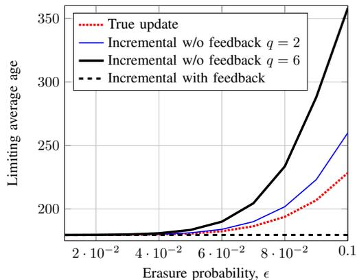
Figure 6. This plot shows the variation of limiting average age as erasure probability  $\epsilon$  increases. We have chosen the number of information bits  $m = 105$ , in each codeword of length  $n = 120$ . The number of bits needed to represent the differential information is taken as  $k = 10$ .
