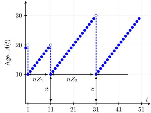
Figure 2. This plot shows one sample path of the age process for the true update scheme. We have taken the codeword length  $n = 10$ . First update sent at time 1 is decoded successfully at time  $n + 1$ , and hence  $Z_1 = 1$ . Second update sent at time  $n + 1$ , fails to get decoded at time  $2n + 1$ , leading to one decoding failure. The following update sent at time  $2n + 1$  is received successfully at time  $3n + 1$ , and hence  $Z_2 = 2$ .
